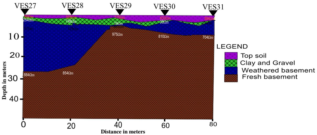
Fig. 9: Goelectrical cross-section along Profile 7.
