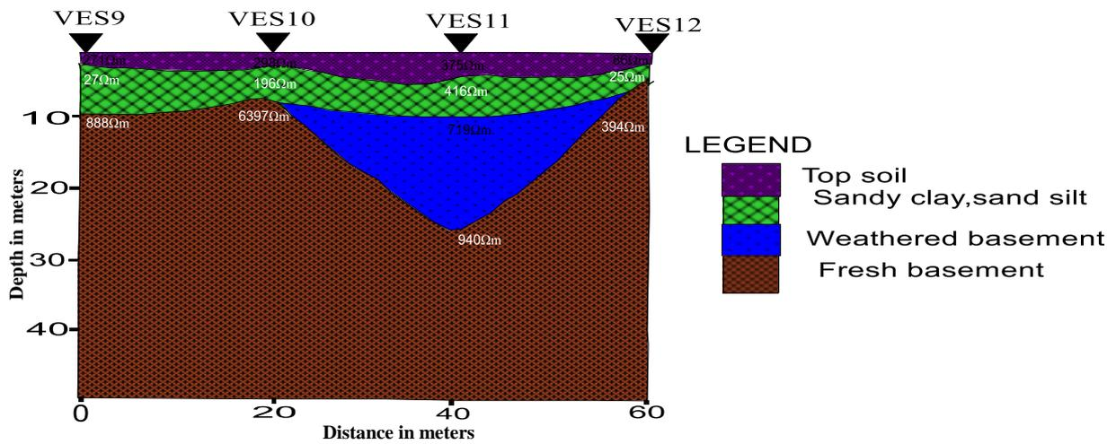
Fig. 5: Geoelectrical cross-section along Profile 3
