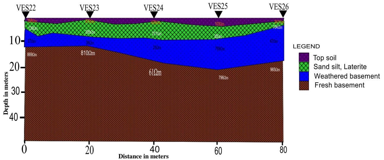
Fig. 8: Goelectrical cross-section along Profile 6.
