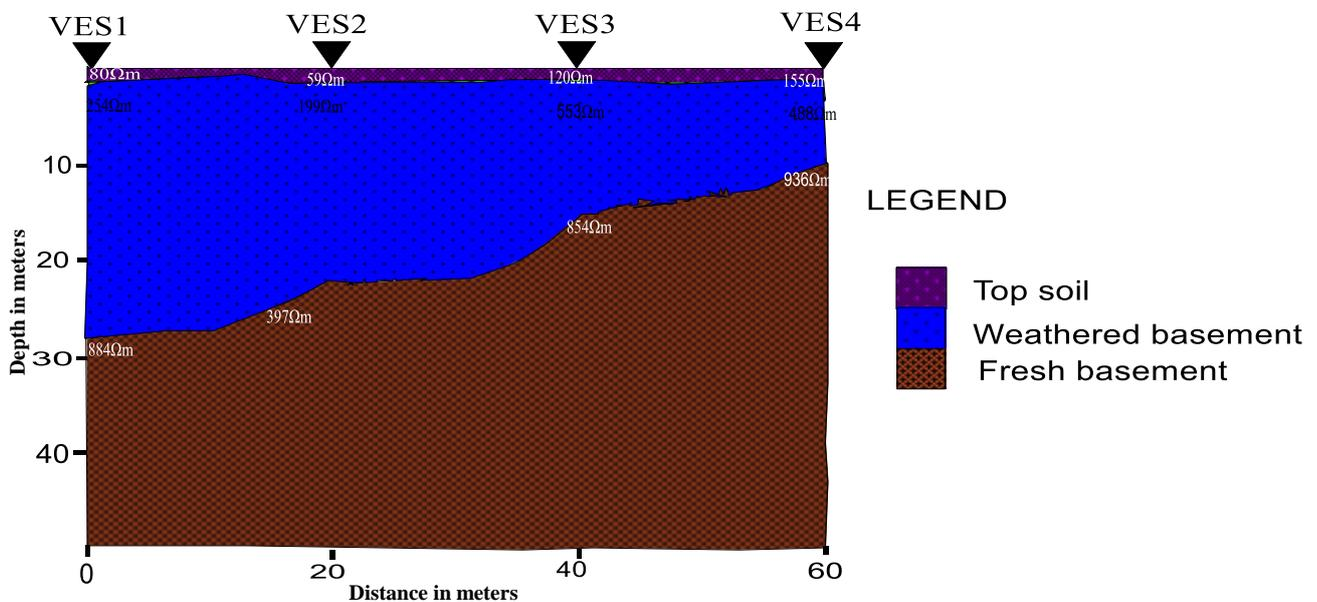
Fig. 3: Geoelectrical cross-section along Profile 1
