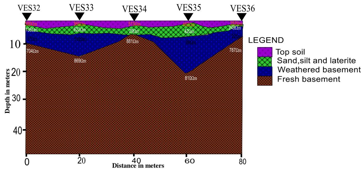
Fig. 10: Goelectrical cross-section along Profile 8.
