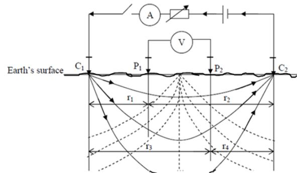
Fig. 2: Current and potential distributions within homogeneous isotropic ground (Telford *et al.*, 1990).
