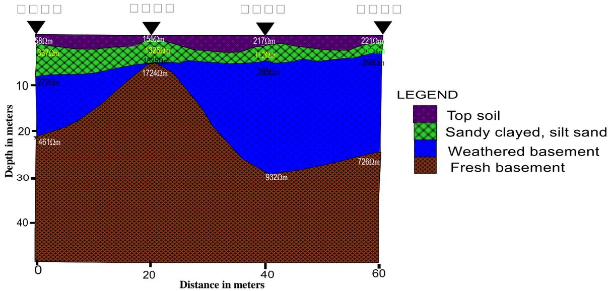
Fig 4: Geoelectrical cross-section along Profile 2
